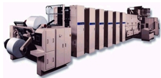
Figure 1. An example of web-handling system: a multi-stage printing machine.
