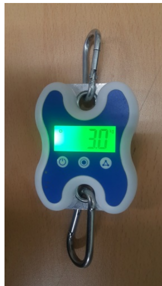
Figure 1. Load-cell type strength-measurement sensor.
