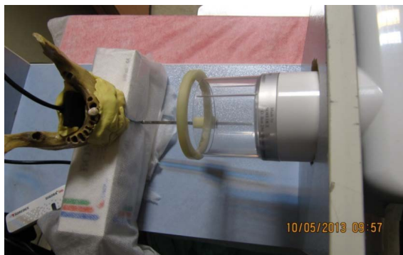
Figure 2. Method of tooth placement in the mandibular socket and X-ray tube adjustment.
