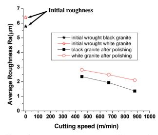
Figure 9. Average roughness, Ra, at different cutting speeds of white and black granite.
