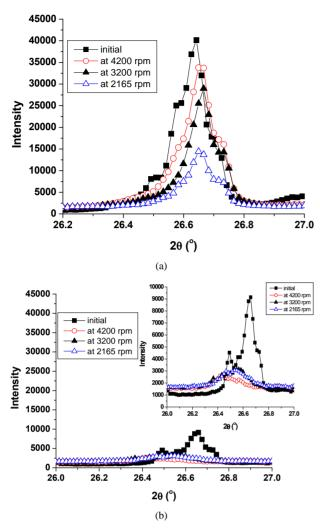
**Figure 7**. XRD diagram at different cutting speed of white and black granite. (a): White granite; (b): Black granite.
