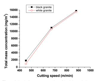
**Figure 6**. Total of mass concentration of Particles emission at different cutting using 60 grit abrasive and 2.5 kg load.
