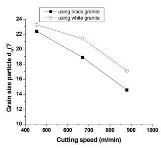
Figure 8. Particle grain size at different cutting speed of white and black granite.
