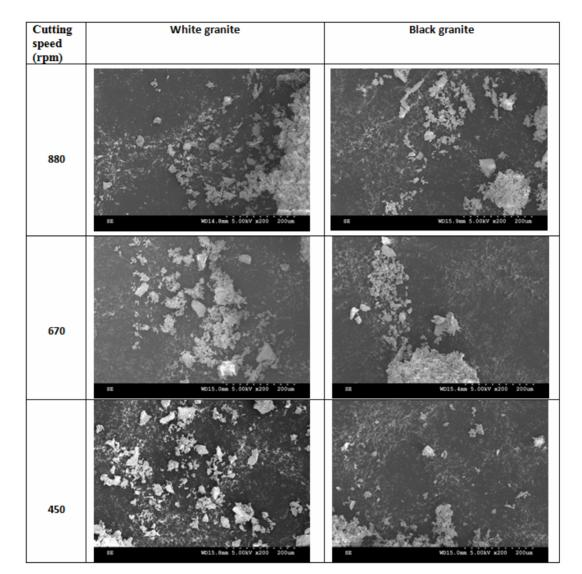
Figure 4. SEM images of particles morphology.
