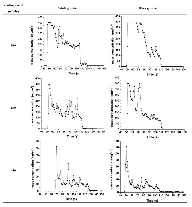
Figure 3. Particles emission at different cutting speed using 60 grit abrasive, 2.5 kg load.
