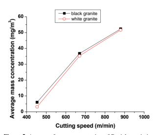
**Figure 5**. Average of mass concentration of Particles emission at different cutting using 60 grit abrasive and 2.5 kg load.
