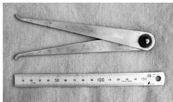
Figure 3. Measuring tools. (Upper) Inside caliper (Shinwa Rules Co. Sanjo, Japan). (Lower) Stainless straight scale (min. unit; 0.5 mm) (JIS QNC08004) (Shinwa Rules Co. Sanjo, Japan).
