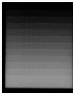
**Figure 2.** Radiographic image of the stepwedge phantom.
