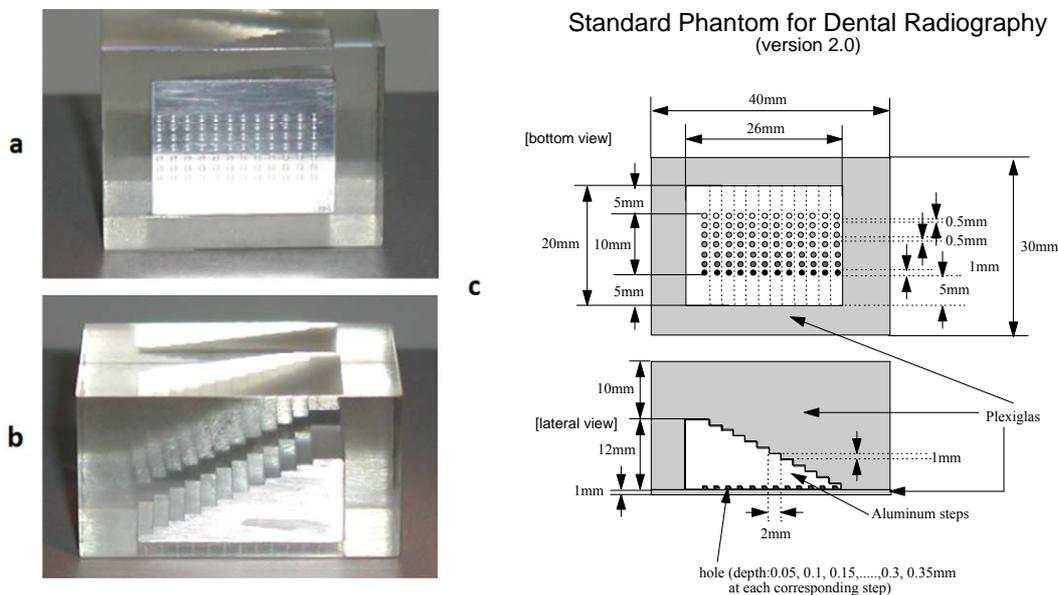
**Figure 1.** Photographs (a,b) and schematic; (c) diagrams of the stepwedge phantom that was used for the evaluation of image quality.
