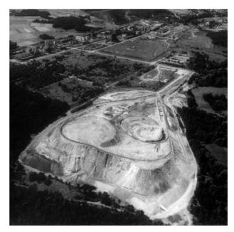
Figure 1. The "Alwernia" Chemical Works—a general view. An active heap of chromic wastes can be seen in the foreground. An old reclaimed heap occupies the area between the factory and the heap.
