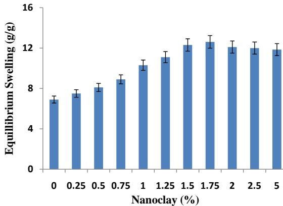
**Figure 6.** Effect of nanoclay on swelling characteristics.
