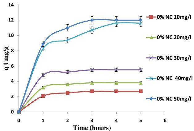
**Figure 10.** Variation of dye adsorption capacity of superabsorbent (without nanoclay) for different initial dye concentration w.r.t contact time.
