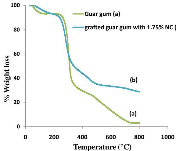
**Figure 4.** TGA thermograms of neat guar gum (a) and grafted guar gum loaded with 1.75% NC (b).
