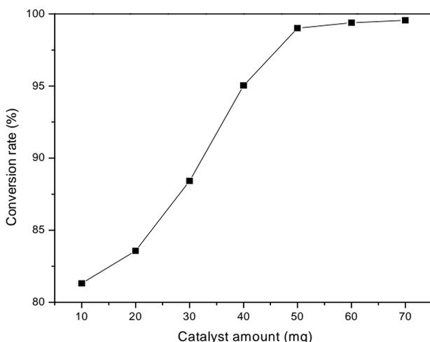
**Figure 7.** Effect of catalyst amount on the esterification of gossypol.
