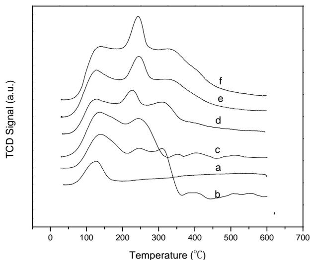
**Figure 4.** NH<sub>3</sub>-TPD curves for a: HMS; b: 20% ZS/HMS; c: 30% ZS/HMS; d: 40% ZS/HMS; e: 50% ZS/HMS; and f: 60% HMS.
