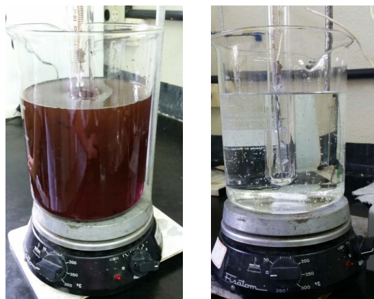
Figure 9. Aspect of the synthetic effluent containing the 4 dyes before and after the application of the photocatalytic treatment with ZnO (2.5 g L -1 in aqueous solution with 8% ethyl alcohol), UV irradiation, temperature-controlled system at 30 °C and pH 10.
