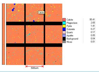
Figure 3. A QEMSCan image of the shale rock sample #33 with a phase analysis shown on the right. The pyrite is designated by yellow color in this image.
