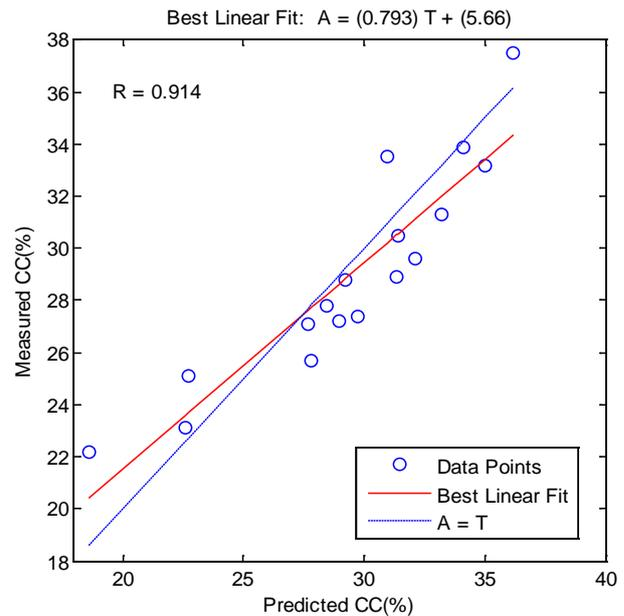
**Figure 3.** ANN prediction versus measured cutting concentration [8,9] for the test data.
