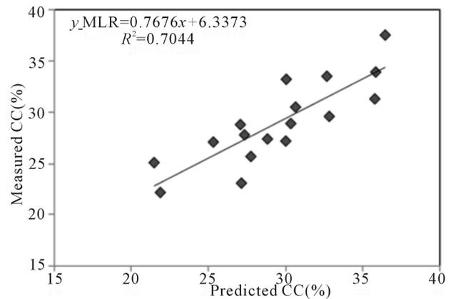
**Figure 6. MLR prediction versus measured cutting concentration [8,9] for the test data.**
