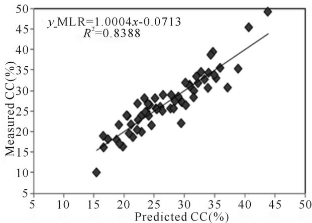
**Figure 5. MLR prediction versus measured cutting concentration [8,9] for the train data.**
