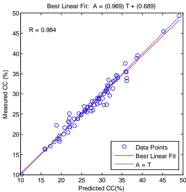
**Figure 4. ANN prediction versus measured cutting concentration (%) for the all data [8,9].**
