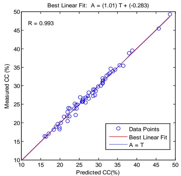
**Figure 2.** ANN prediction versus measured cutting concentration [8,9] for the training data.
