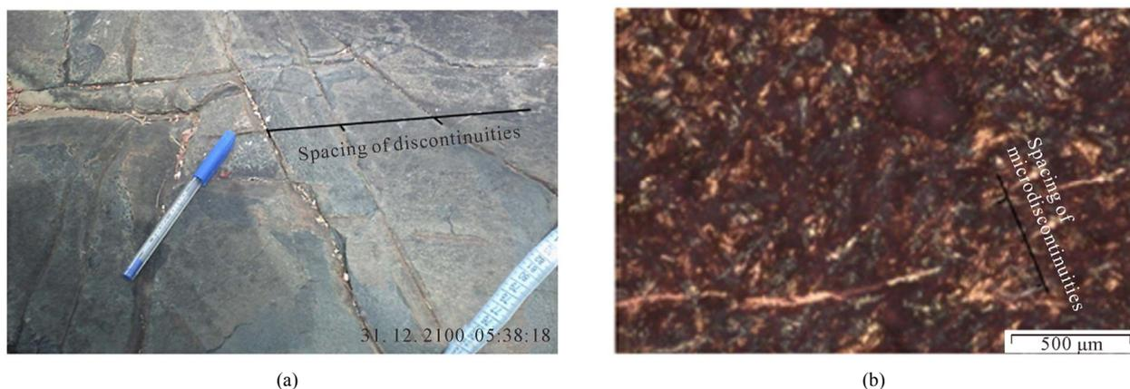
Figure 12. Fractal analysis of spacing of discontinuities ((a) outcrops scale; (b) preparation scale).
