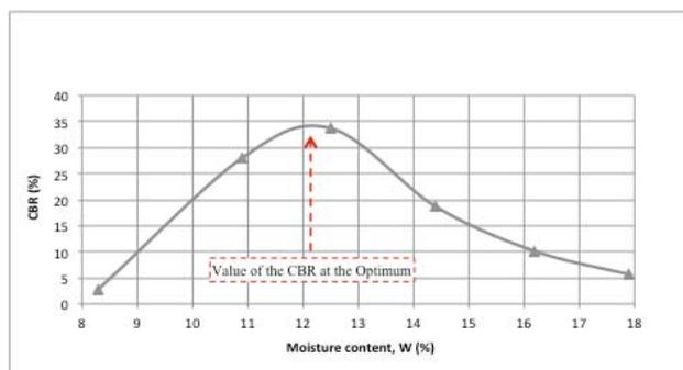
**Figure 3. The CBR obtained from the Optimum of the Moisture content (the standardized method).**
