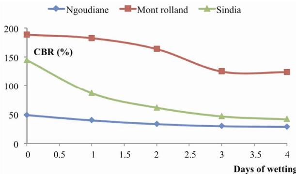
Figure 7. Evolution of the CBR with the days of immersion.
