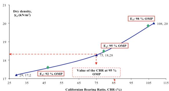
**Figure 2. An example of the West African Compaction (WAC) method of determination of the CBR.**
