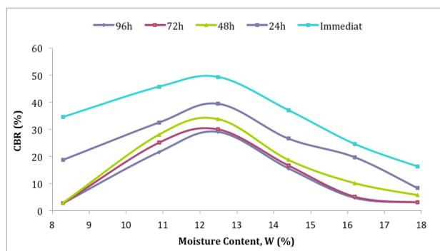
**Figure 4. CBR versus moisture content according to time of immersion (Ngoundiane).**
