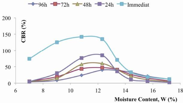
Figure 5. CBR versus moisture content according to time of immersion (Sindia).
