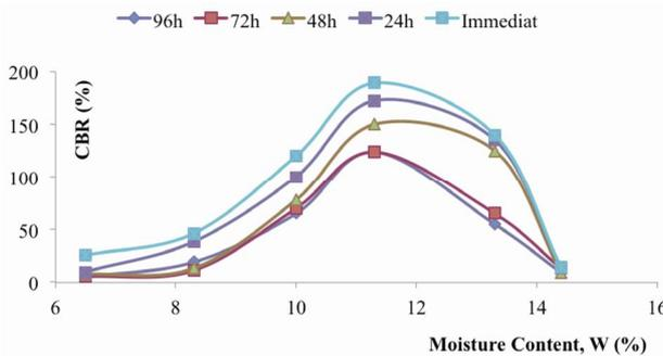
Figure 6. CBR versus moisture content according to time of immersion (Mont-Rolland).
