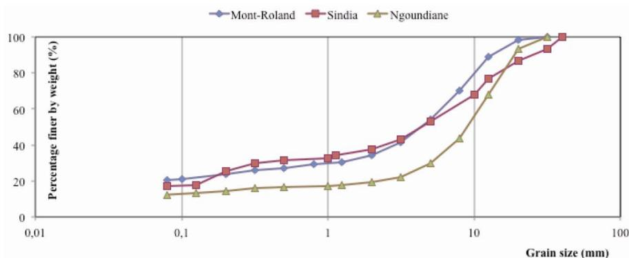
Figure 1. Grain size distribution of the gravel lateritic soils.
