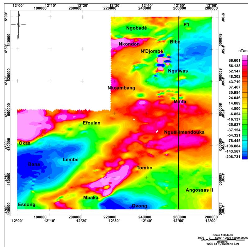
Figure 5. Total magnetic intensity anomaly map reduced to equator. Line P1 corresponds to the profile selected for modeling.
