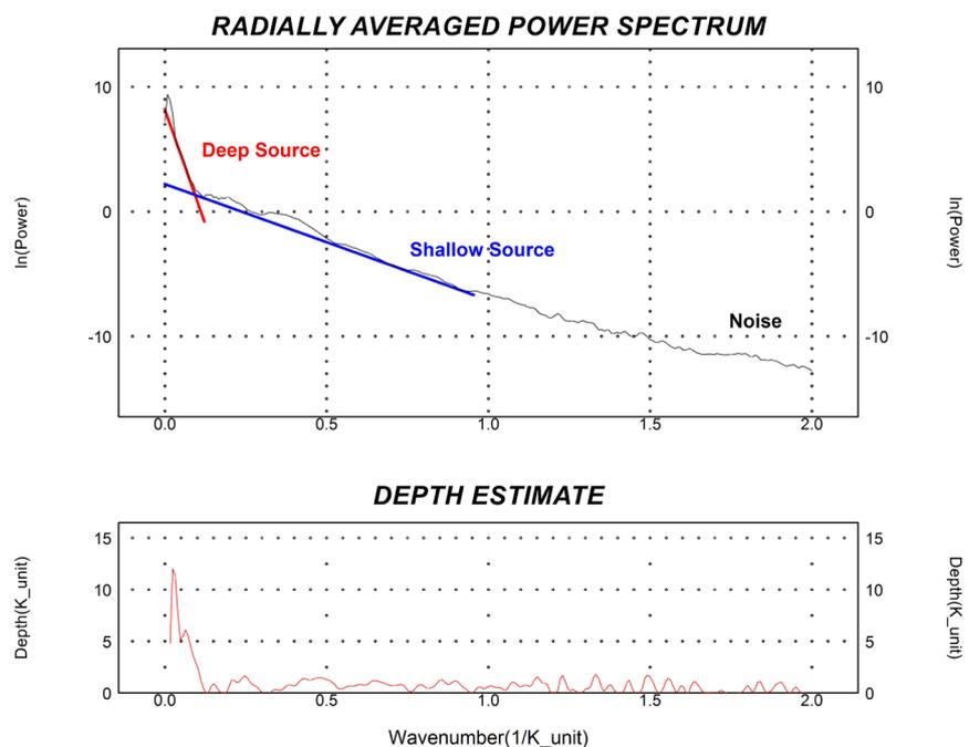
**Figure 8.** Power spectrum showing the mean depth to the basement rock in the study area.
