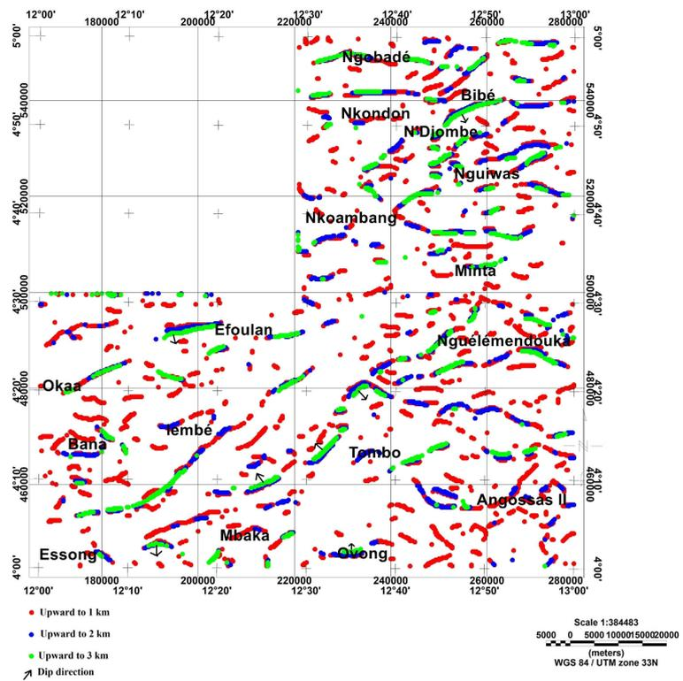
**Figure 2.** Superposition of maxima of horizontal gradient of TMI-RTE upward continued to 1 km, 2 km and 3 km (Mono et al., 2018b).
