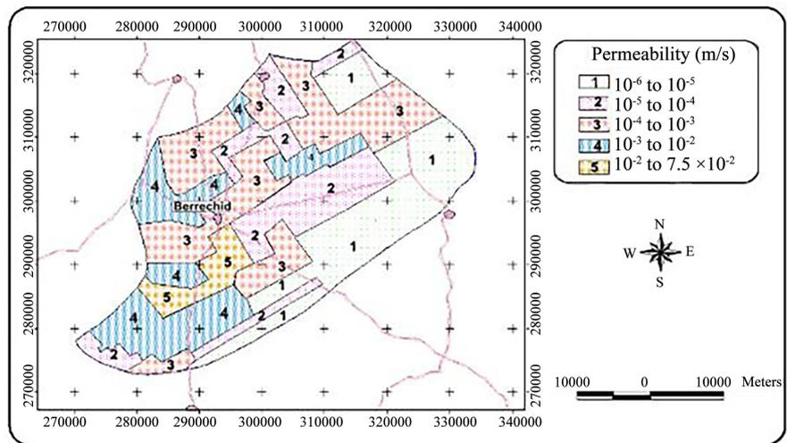
Figure 4. Distribution of the permeabilities resulting from steady-state calibration.
