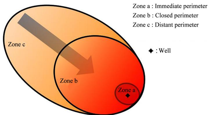
**Figure 2.** Presentation of perimeters of protection around a pumping well.
