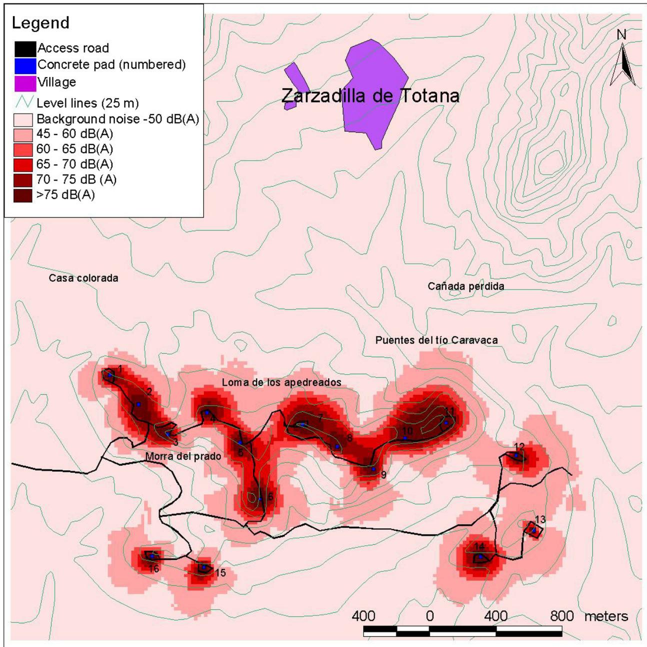
**Figure 5.** Noise map in operation phase: maximum power.
