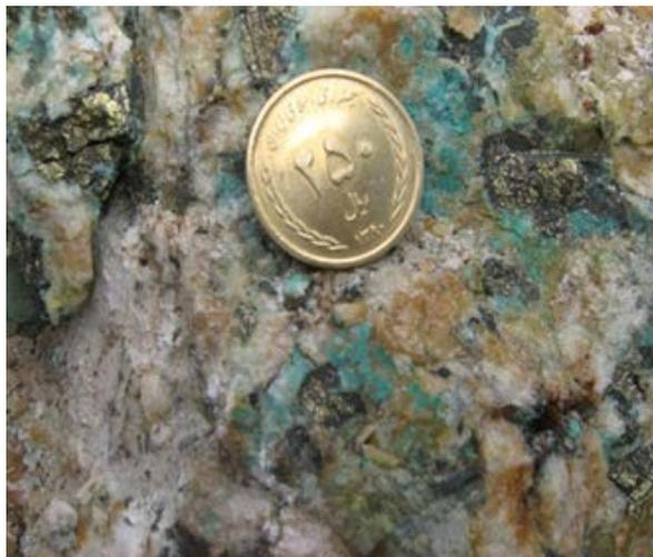
**Figure 29.** Oxide mineralization associated with the fault and presence of iron oxides in hosting polygenetic conglomerate rock.
