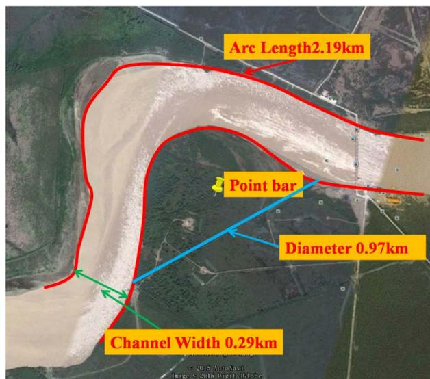
**Figure 5.** Schematic diagram of measuring point bar's parameters of the Yellow River. The red line is the arc length. The yellow landmark is the position of the point bar. The green arrow is the channel width. The blue line is the diameter of the point bar.
