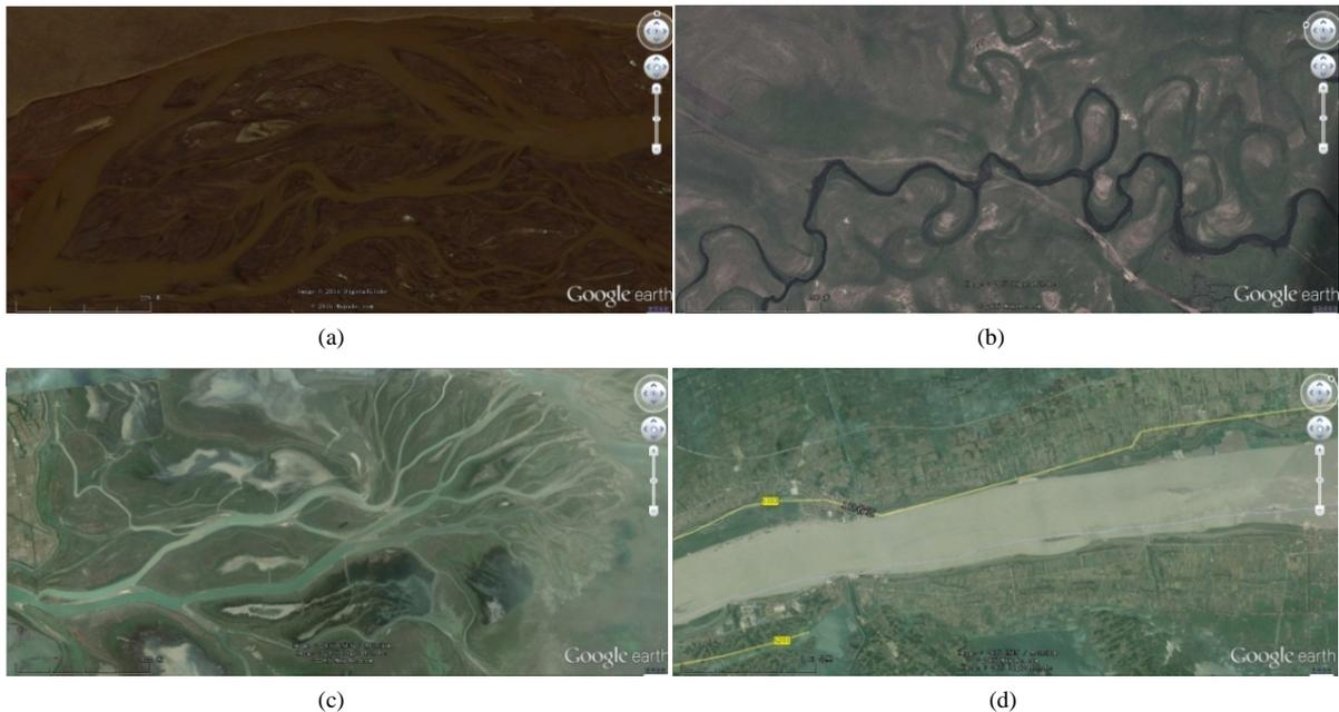
**Figure 1.** Satellite’s image of different types of river. (a) Braided river has many channel bars in the whole valley and its channel branches off around diara; (b) Meandering River has features of single channel, high curvature, low terrain slope; (c) Anastomosing River has features of multi-channel, straight or curved, and has stable riverbank composed of fine-grained sediments (silt or clay) and vegetation; (d) Straight River has features of single channel, low curvature.
