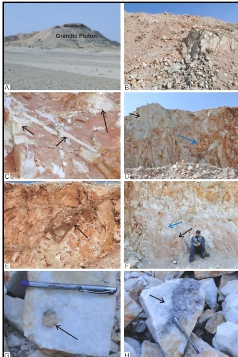
Figure 2. Shows (A) General view of Rod El Leqah quartz body capping granitic pluton; (B) Pale pink granite host rock; (C) Rafts from granite enclosed within quartz body; (D) Extraction face of quartz appears in milky white color and change to red due to iron oxide staining along fractures and fissures (blue arrow); (E) Lenticular sheet of iron oxide within highly deformed zone in the quartz body (black arrow); (F) Mélange of quartz and feldspars (black arrow); (G) Xenocryst of feldspar within quartz fragments; (H) Opaque minerals and mica associated with the quartz body.
