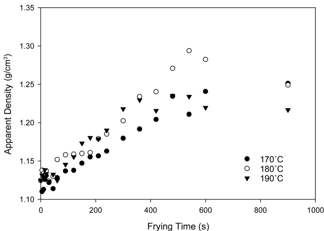
**Figure 2.** Apparent density as a function of time for de-boned chicken meat deep-fat fried at 170°C, 180°C, and 190°C.
