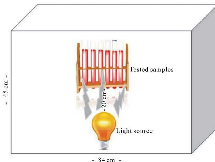
Figure 1. Chamber shows light source and distance to the tested sample.
