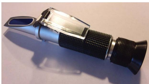
**Figure 1.** Hand-held optical refractometer.
