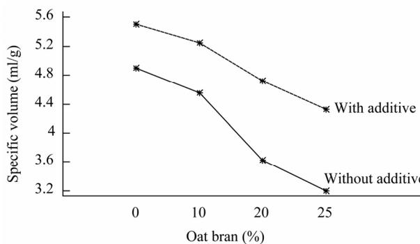
**Figure 2. Specific volume (ml/g) as a function of oat bran and additive.**
