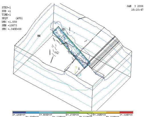
**Figure 6. Average principal stress contour when B901 face mining was over.**
