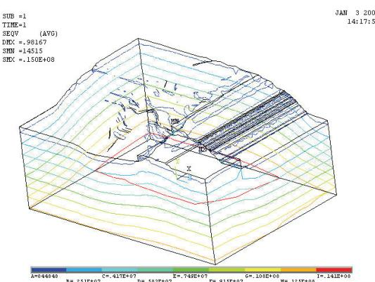
**Figure 5. Average principal stress contour in original state.**
