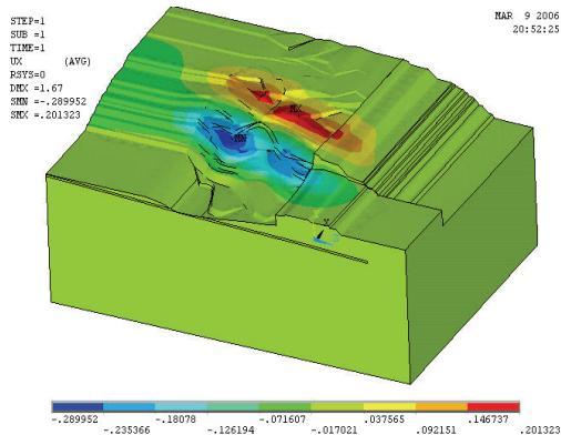
**Figure 4. X direction displacement when B901 face mining was over.**
