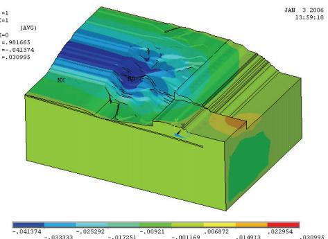
**Figure 3. X direction displacement in original state.**
