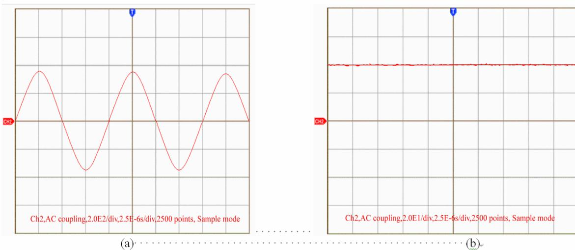
Figure 18. Experimental results for series parallel resonant converter at 60% load with  $m=1$ : (a)  $V_{Ls}$ , (b)  $V_0$  with filter.
