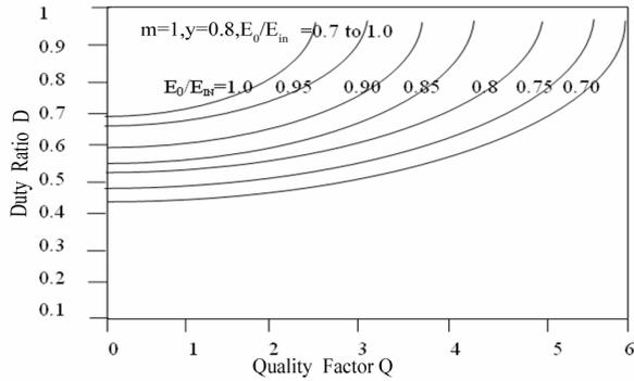
Figure 10. Variation of duty ratio versus quality factor with  $m = 1, y = 0.80$ .
