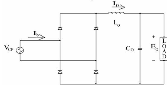
Figure 3. Output circuit of bridge rectifier and filter component to resonant converter.
