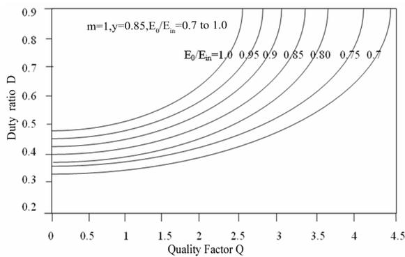
Figure 11. Variation of duty ratio versus quality factor with  $m = 1, y = 0.85$ .
