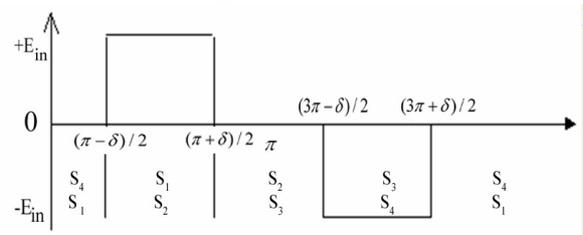
Figure 4. Quasi-square voltage waveform of LCC resonant converter.
