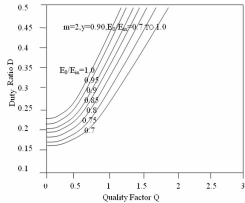
Figure 16. Variation of duty ratio versus quality factor with  $m = 2$ ,  $y = 0.90$ .
