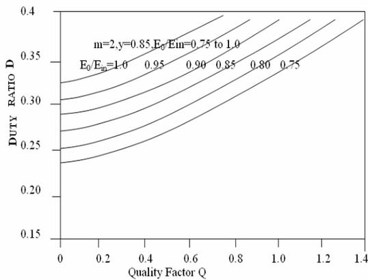
Figure 15. Variation of duty ratio versus quality factor with  $m = 2$ ,  $y = 0.85.5$ . Design of series parallel resonant converter.
