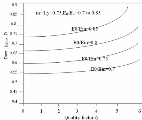
Figure 9. Variation of duty ratio versus quality factor with m = 1, y = 0.75.
