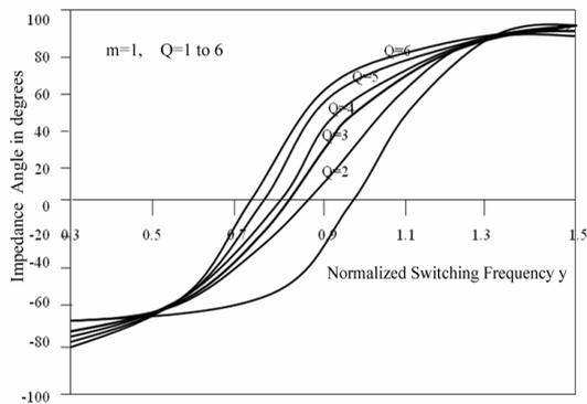
Figure 7. Variation of impedance angle in degrees versus normalized switching frequency for various values of Q with m = 1.
