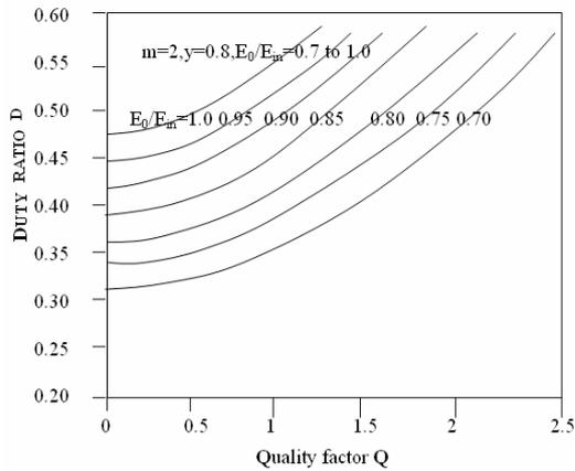
Figure 14. Variation of duty ratio versus quality factor with  $m = 2$ ,  $y = 0.80$ .
