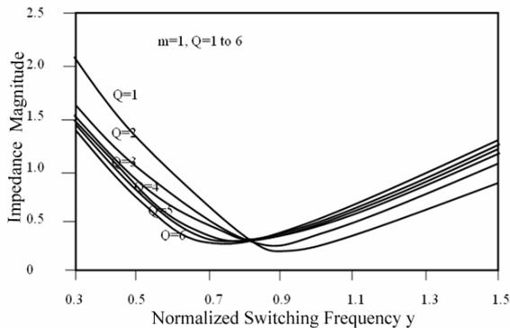
Figure 6. Variation of impedance magnitude versus normalized switching frequency for various values of Q with m = 1.
