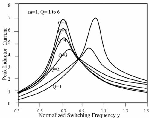
Figure 8. Variation of peak inductor current versus normalized switching frequency for various values of Q with m = 1.
