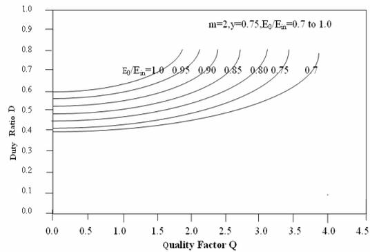
Figure 13. Variation of duty ratio versus quality factor with  $m = 2, y = 0.75$ .
