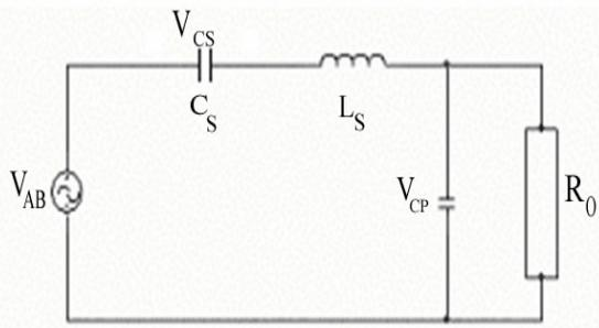
Figure 5. AC equivalent circuit of resonant converter.
