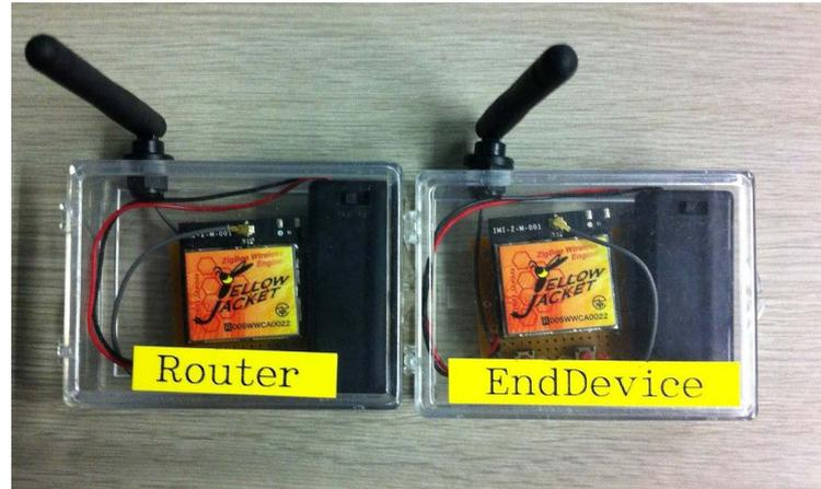
Figure 7. Images of the ZED and the ZR devices (IMI-Z-M-001).
