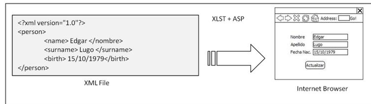
Figure 5. Diagram of a method for editing an XML file with XSLT and ASP.
