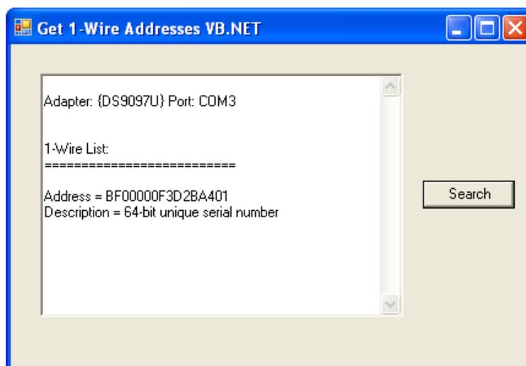
**Figure 8.** Results of identifying an iButton with the testing software.
