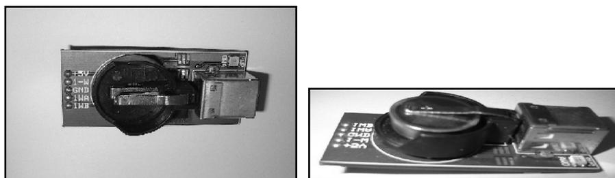
**Figure 7.** Hardware interface for exchanging information between a PC and the iButton.
