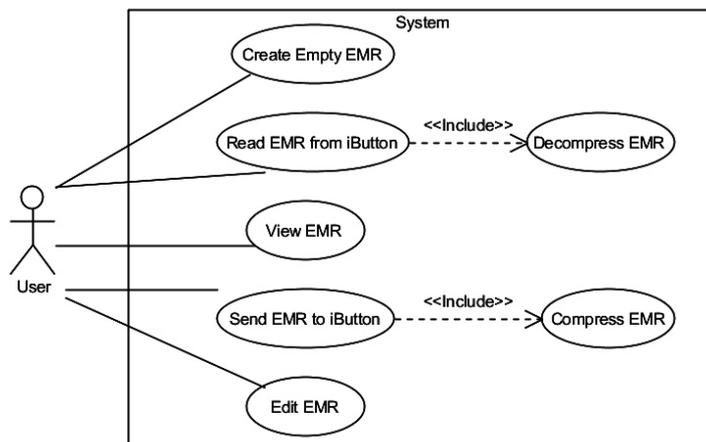
**Figure 2.** UML use case diagram for the EMR managing system.
