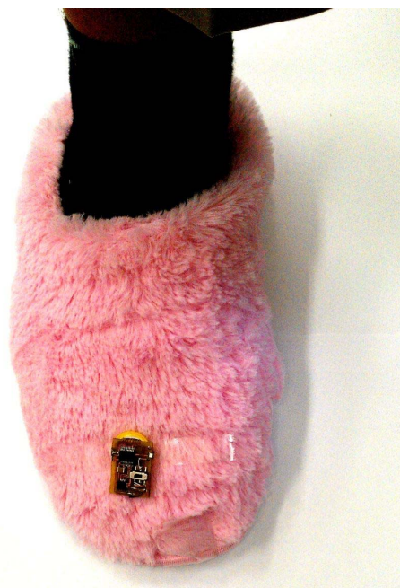
Figure 4. BEAT sensor attached to a slipper worn by a healthy volunteer.
