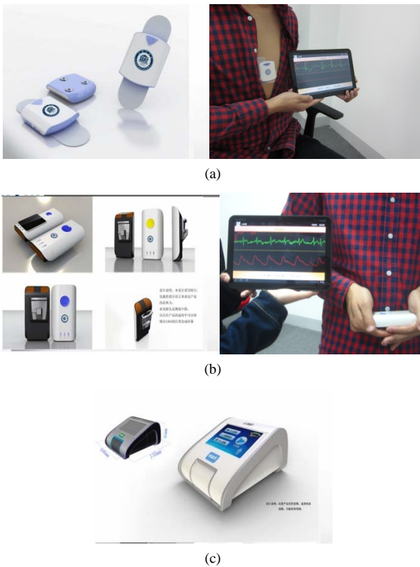
Figure 2. Body Sensors for different applications. (a) Mini-Holter; (b) 3-in-1 Portable Monitor; (c) Intelligent Sphygmomanometer.
