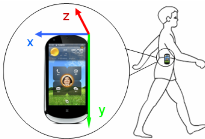
Figure 2. The position of wear mobile phone and the coordinate of fall detect system.
