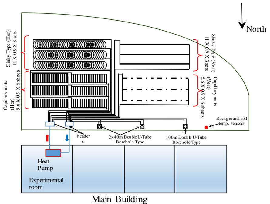
**Figure 2.** Schematic showing the configuration of heat exchangers in the test field.
