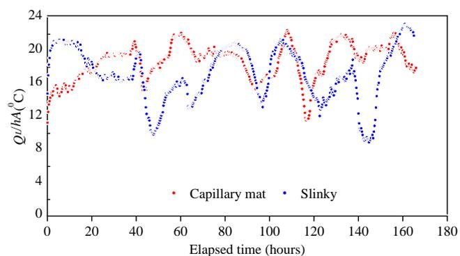
**Figure 14.** Calculated heat load for the both experiments using capillary mats and slinky heat exchangers.
