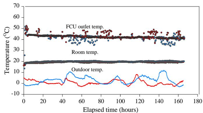
**Figure 11.** Outdoor temperatures, room temperatures and Fan Coil Unit (FCU) air temperatures for both slinky and capillary mats heat exchangers.
