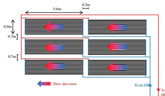
**Figure 5.** Schematic arrangement of the capillary mat heat exchangers.
