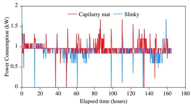
**Figure 13.** Electricity consumption for both capillary mat and slinky heat exchanger.
