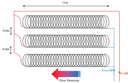
Figure 6. Schematic arrangement of the slinky heat exchangers.
