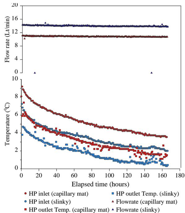
**Figure 10.** Heat-pump inlet and outlet temperatures and volumetric flow-rate of ground heat exchanger fluid.
