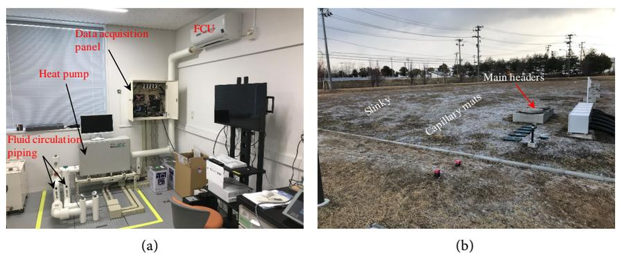
**Figure 3.** Experimental room with the main GSHP system (a) and installation area of GHE's (b).
