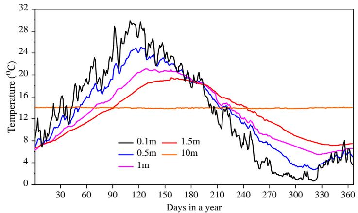
**Figure 1.** Annual soil temperature recorded at the test site, from April 1, 2018 to March 31, 2019.
