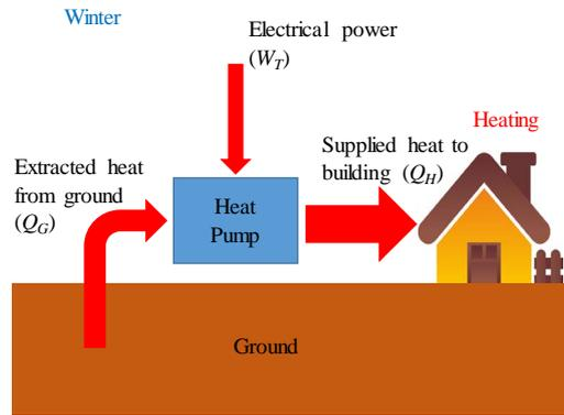
**Figure 9.** Schematic of energy flow during space heating using GSHP.
