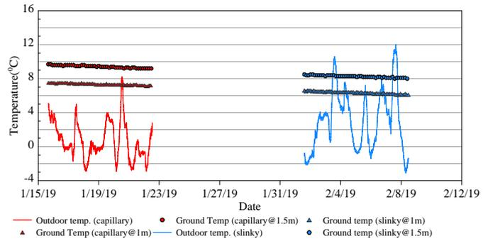
Figure 7. Outdoor temperature and ground temperatures at 1 m and 1.5 m depths, during experimental periods.
