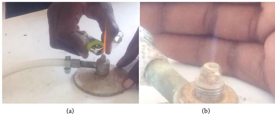
**Figure 4.** Flammability test set-up. (a) Propagation of the flame; (b) Complete combustion of the biogas.
