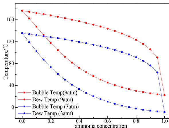
**Figure 9.** Influence of ammonia concentration on the dew and bubble temperature.
