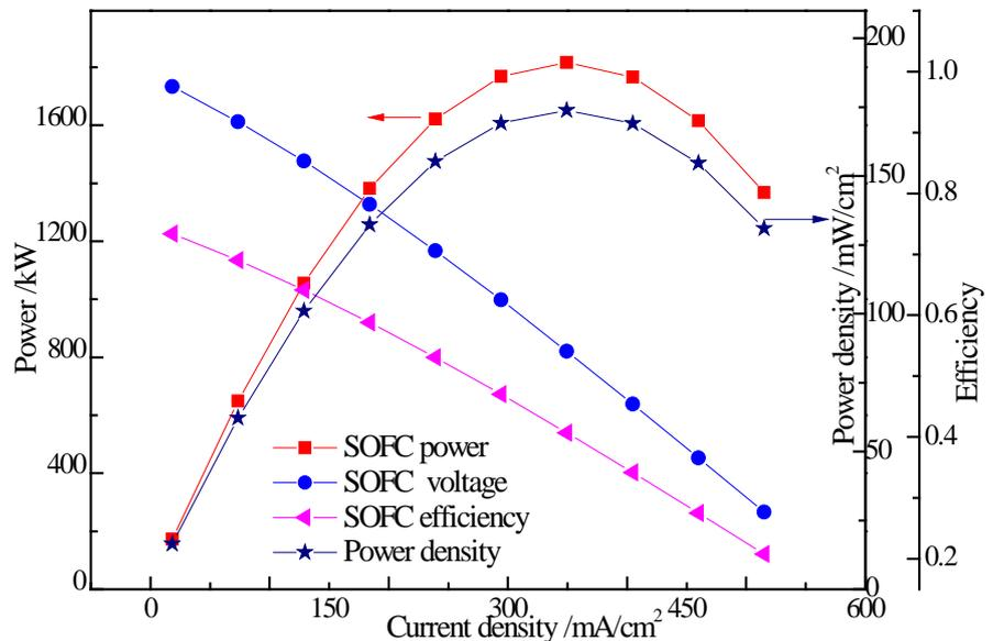
**Figure 6.** Influence of current density on the performance of the system.
