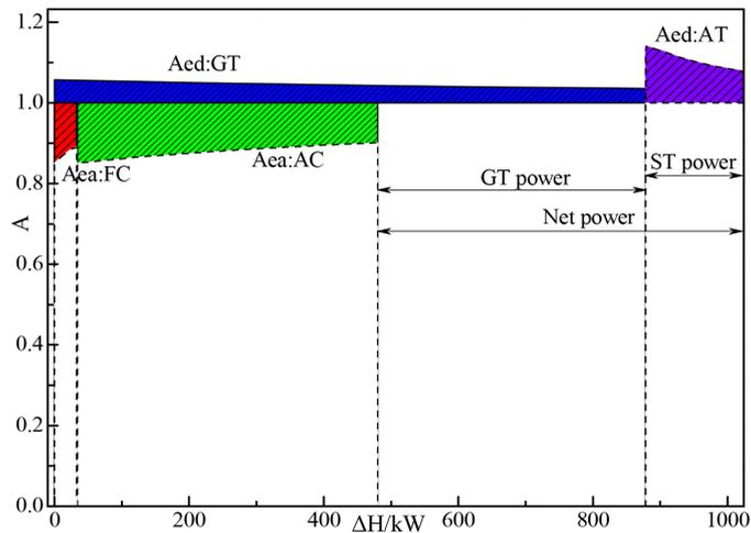
**Figure 12.** Energy-utilization diagram (EUD) of the power blocks.
