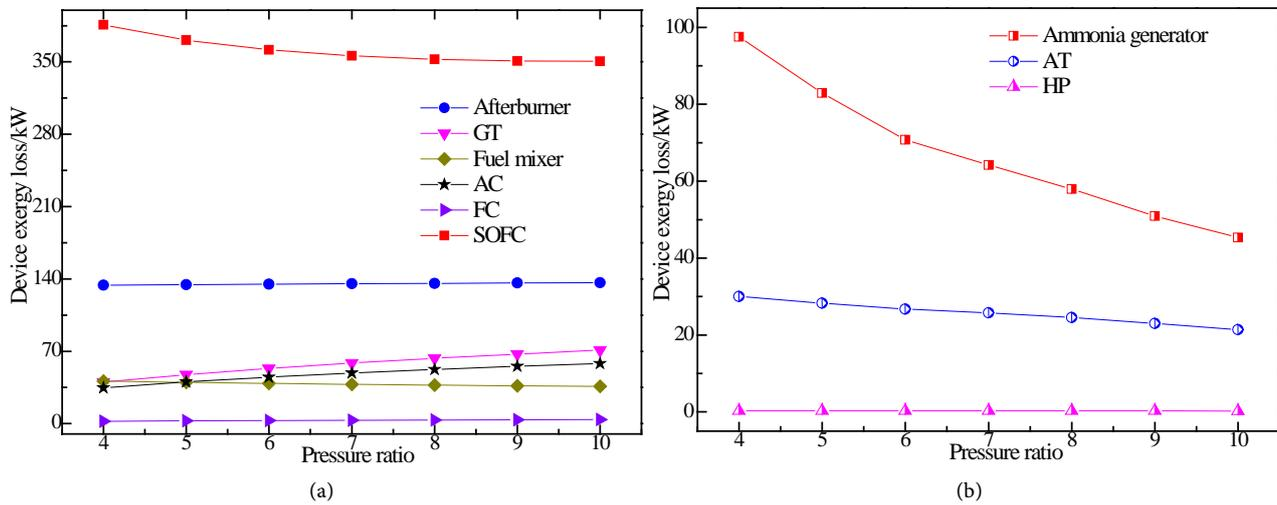
**Figure 4.** Effects of compressor pressure ratio on the energy destruction in each component.
