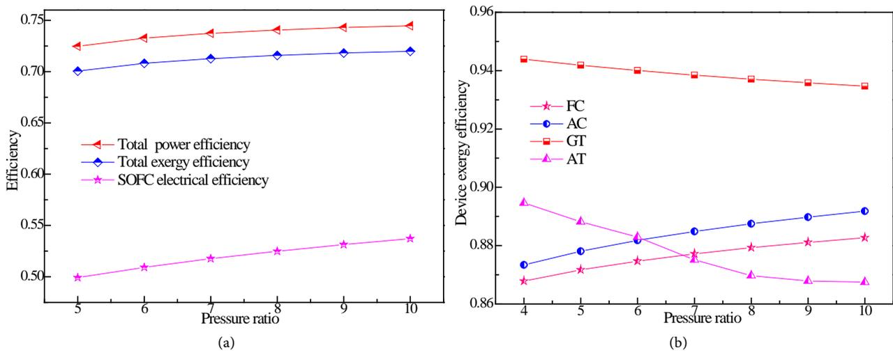
**Figure 5.** Effects of compressor pressure ratio on the efficiency of system and each component.
