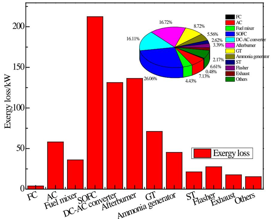
**Figure 3.** Exergy destruction of each component in SOFC-GT-Kalina system.
