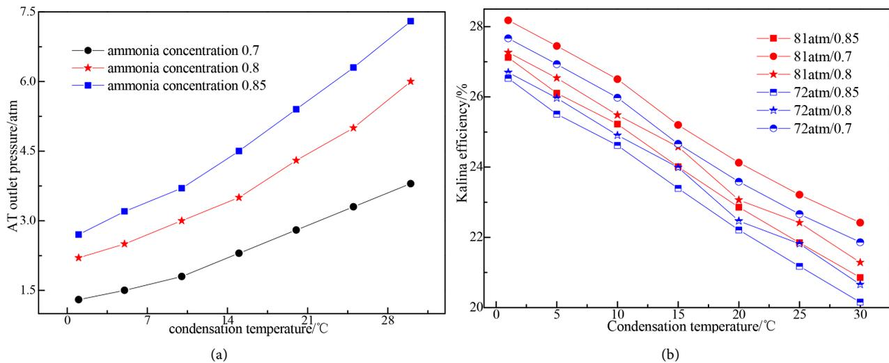
**Figure 10.** Influence of condensation temperature on the performance of the system.
