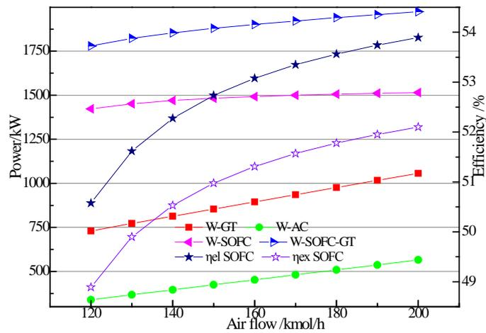
**Figure 7.** Influence of air mass flow on the performance of the system.
