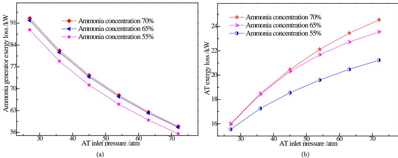
**Figure 8.** Influence of AT inlet pressure and ammonia concentration on the exergy destruction of main components.
