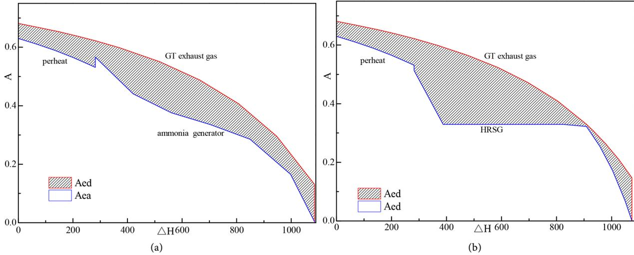
**Figure 11.** Energy-utilization diagram (EUD) of heat exchange processes.
