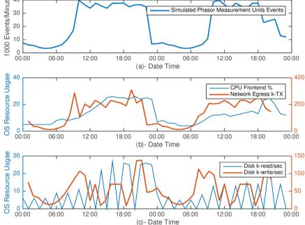
Figure 4. (a) shows a simulation data of a Phasor Measurement Units (PMU) recording device workload. (b) and (c) shows a normal system usage patterns, CPU, network and Disk usage respectively.
