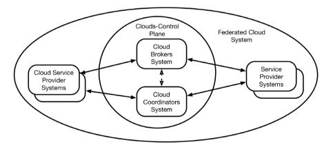
**Figure 2.** Proposed Federation of Power System CSP's, dedicated as s SoS includes cloud service providers and energy service providers. The Clouds-Control plane Clouds-Broker and Clouds-Coordinator.
