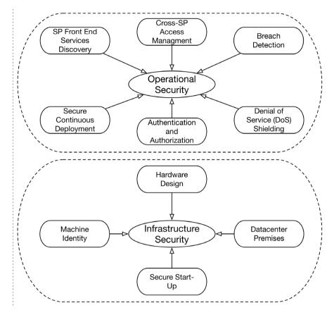
**Figure 1.** Federation of Power System CSP's security design. Comprises of infrastructure security and operational security layers.
