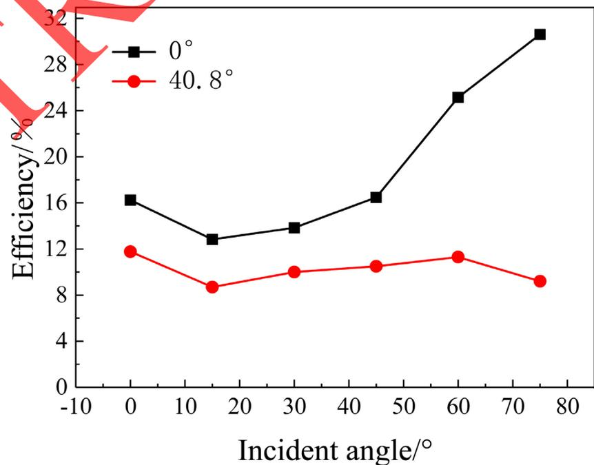
**Figure 3.** Variation of optical efficiency at different latitudes.
