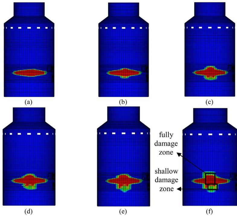
**Figure 5.** Condition I: Damage propagation process. (a) 5 ms. (b) 10 ms. (c) 20 ms. (d) 30 ms. (e) 40 ms. (f) 50 ms.
