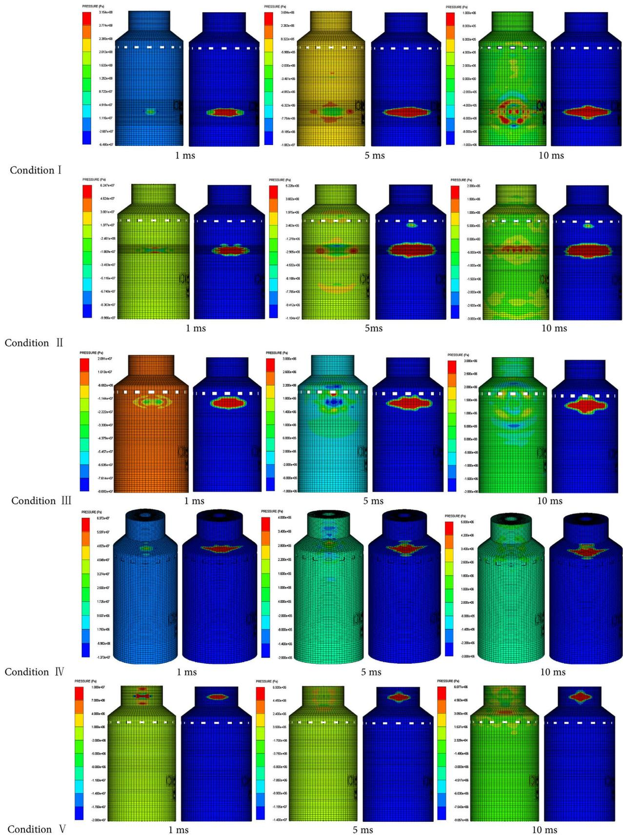
Figure 7. Comparison of pressure and damage cloud of condition I, II, III, IV, V.
