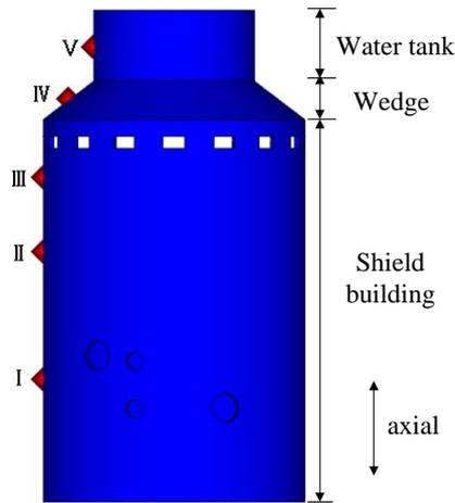
**Figure 2.** The arrangement of the burst spot.
