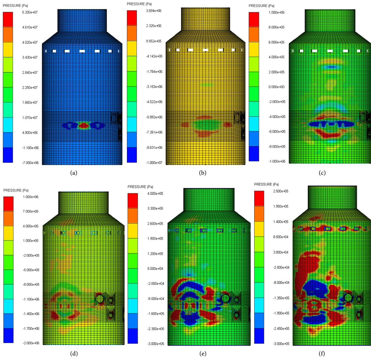
**Figure 4.** Condition I: Time sequences of pressure wave (Pa). (a) 1 ms. (b) 5 ms. (c) 9 ms. (d) 20 ms. (e) 30 ms. (f) 50 ms.
