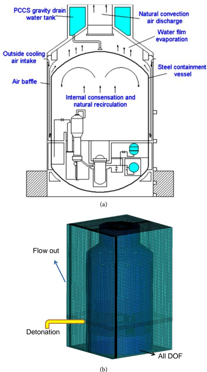
**Figure 1.** Model of an AP1000 shield building. (a) Geometry of the shield building. (b) Fully coupled numerical model and the boundary conditions.
