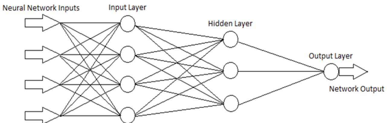
**Figure 1.** Artificial neural network architecture.
