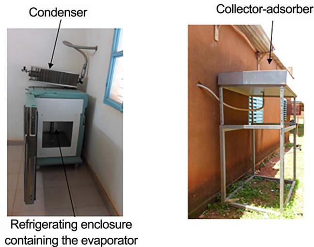
**Figure 2.** Photography of solar adsorption refrigerator.
