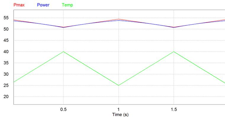
Figure 2. Power tracker response under temperature variations. Top traces: superimposed signals P<sub>max</sub> and extracted Power. Bottom trace: temperature profile applied.
