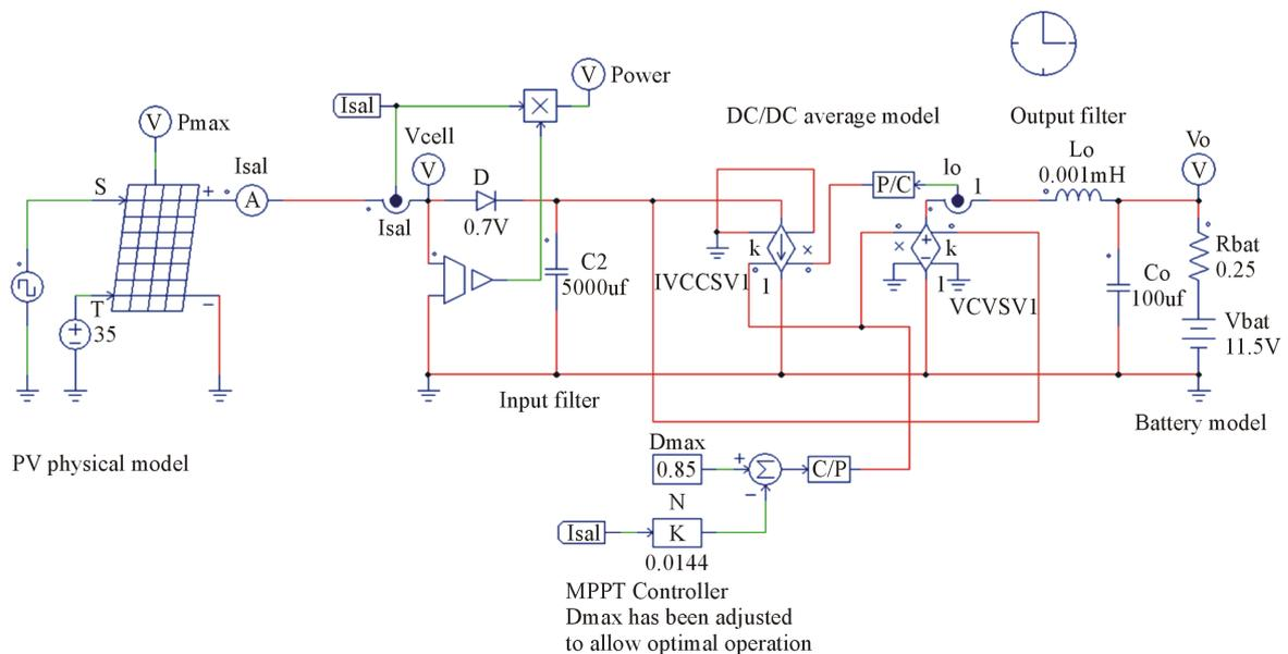
Figure 1. PSIM diagram used to simulate the MPPT-PV with feedback-current.
