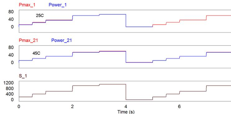
**Figure 5.** Staircase function as incoming signal over S terminal available in solar cell model. Simultaneously, a parameter sweep analysis is used in order to produce temperature variations considering a range between 25°C to 45°C.
