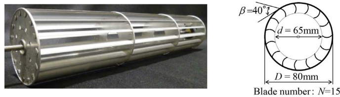
Figure 2. Cross-flow wind turbine.
