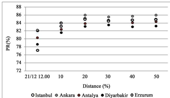
**Figure 6.** The performance ratio related to the row distance.
