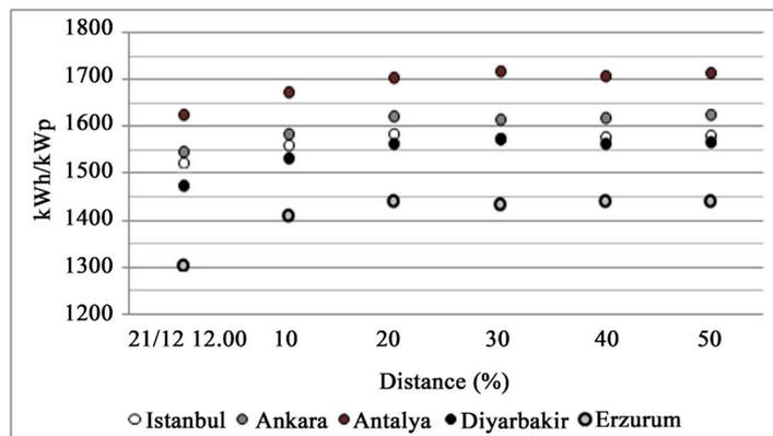
**Figure 5.** The final PV system yield related to the row distance.
