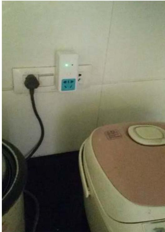
**Figure 7.** Actual picture of smart socket.
