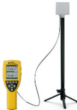
Figure 1. the EHP50C probe connected to the NBM550 meter through a fiber cable.
