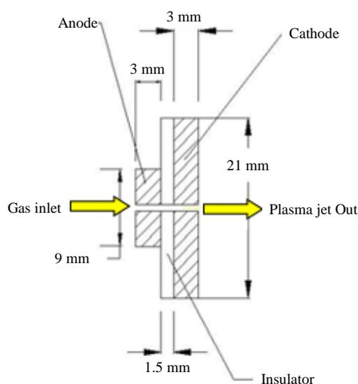
**Figure 1.** Schematic diagram of electrode system of the ANPJ device.
