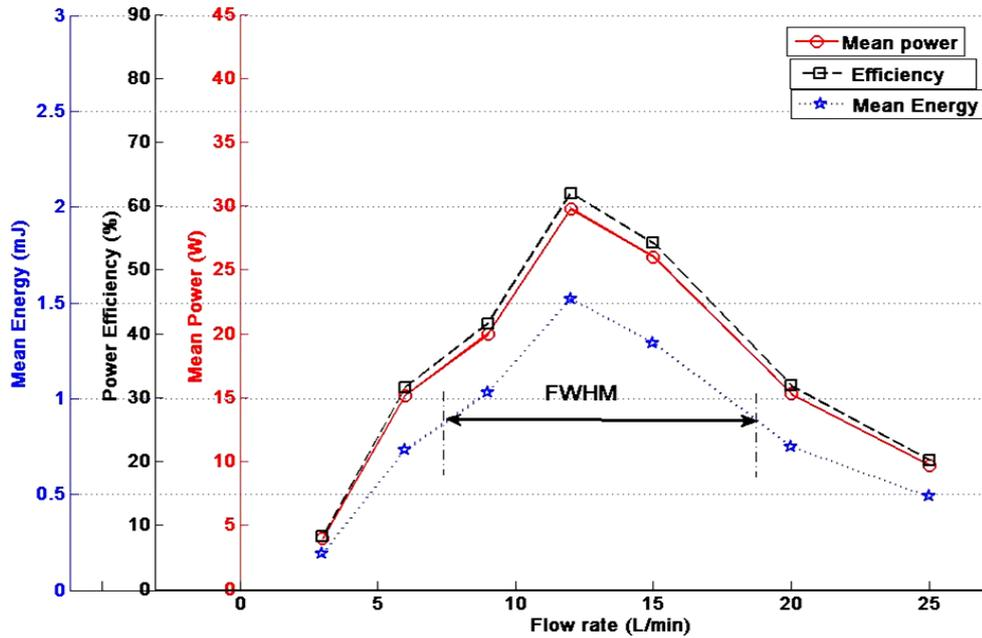
Figure 10. The mean power, power efficiency and mean energy versus the different N<sub>2</sub> gas flow rates.
