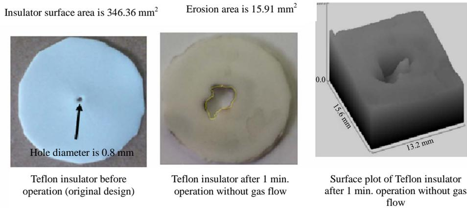
**Figure 12.** Photograph of the Teflon insulator before operation and after 1 min operation without gas flow.
