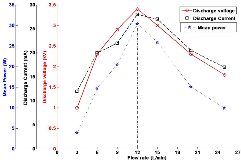
**Figure 8.** The discharge voltage, discharge current and consumed power (traditional method) versus different N<sub>2</sub> gas flow rates.
