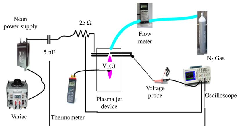
**Figure 4.** Experimental arrangement and the diagnostic techniques of ANPJ device.
