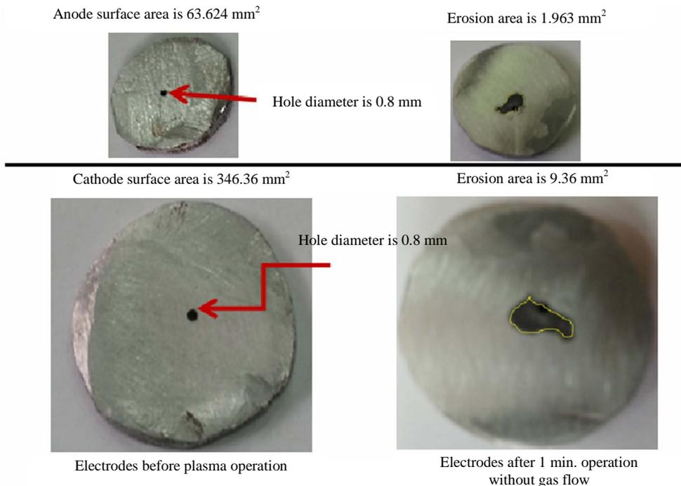
**Figure 13.** Photograph of the Electrodes before operation and after 1 min operation without gas flow.
