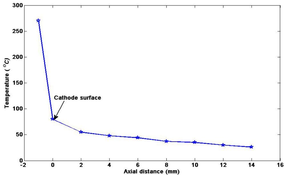
Figure 11. The gas temperature versus the different axial distances of N<sub>2</sub> plasma jet at 12 L/min flow rate.
