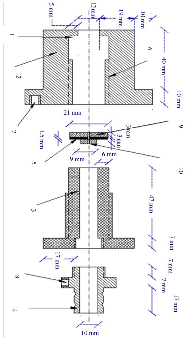
**Figure 2.** Construction drawing of ANPJ device.
