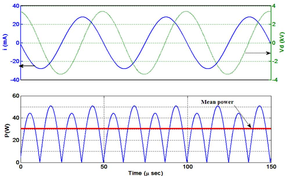
**Figure 7.** The discharge voltage, discharge current and consumed power with N<sub>2</sub> gas flow rate of 12 L/min.
