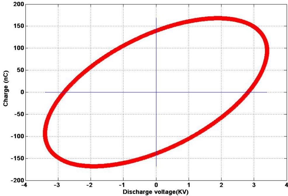
**Figure 9.** Lissajous figure for the ANPJ device at  $N_2$  gas flow rates of 12 L/min and at 6 kV input voltage.
