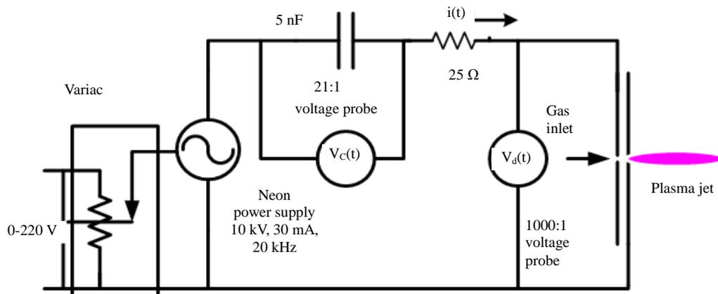
**Figure 3.** The electric circuit of the ANPJ device.
