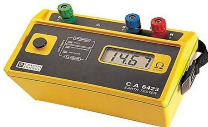
[Figure 1](#). C.A. 6423 Digital Earth Tester.
