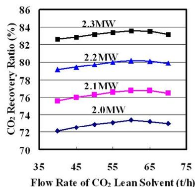
**Figure 3.** CO<sub>2</sub> recovery ratio as functions of flow rate of CO<sub>2</sub> lean solvent and reboiler duty.
