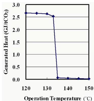
Figure 6. Generated heat as a function of operation temperature at 101.3 kPa.
