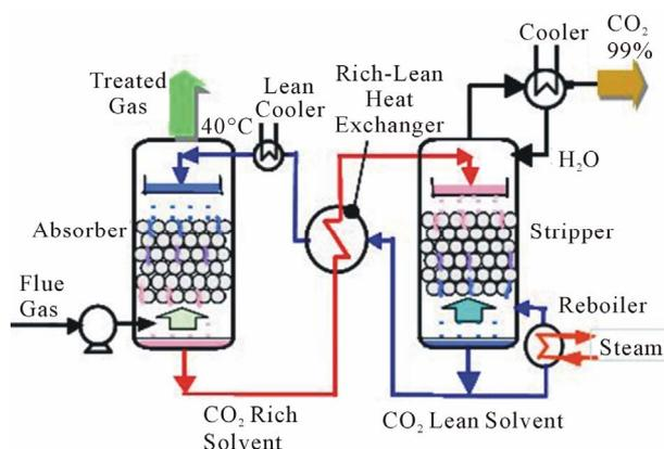
**Figure 1. Carbon dioxide capture system.****Table 2. Design conditions of CO<sub>2</sub> capture system.**
