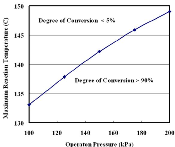
Figure 7. Maximum reaction temperature as a function of operation pressure.
