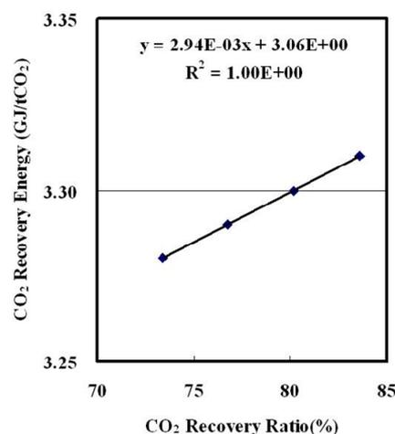
**Figure 4.** CO<sub>2</sub> recovery energy as a function of CO<sub>2</sub> recovery ratio.
