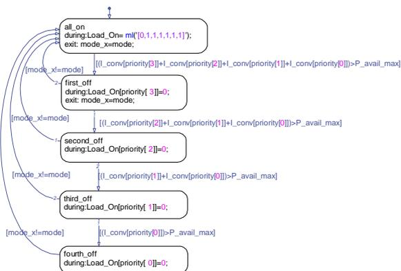
**Figure 13. Algorithm for the load management.**
