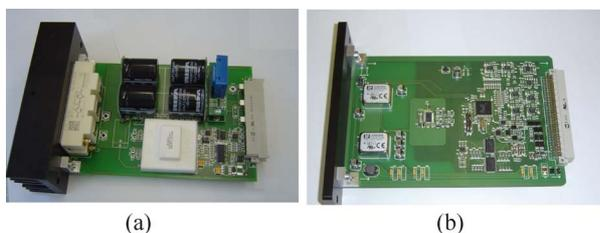
**Figure 3. (a) Power module, (b) DSP module.**
