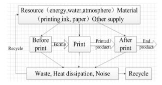
Figure 3. Material flow in the process of printing.
