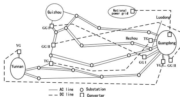
Figure 1. CSG grid structure framework in 2010.
