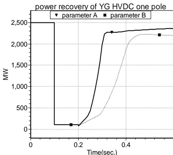
**Figure 3. YG HVDC mono-polar power restoration comparison curve under parameters A and B.**
