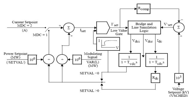
**Figure 2. Diagram of DC model CDC6T.**
